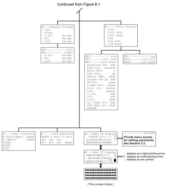
Figure 8-2 The TLS Maintenance Menu (Part 2)
